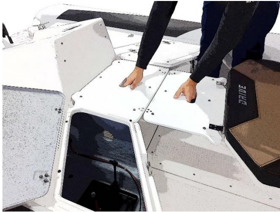
Fig. 47. How the rear sundeck should be installed.
