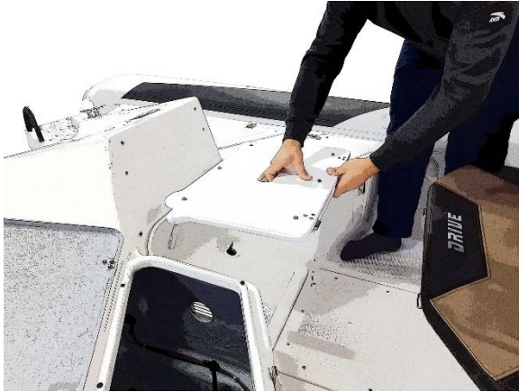
Fig. 46. How the rear sundeck should be installed.
