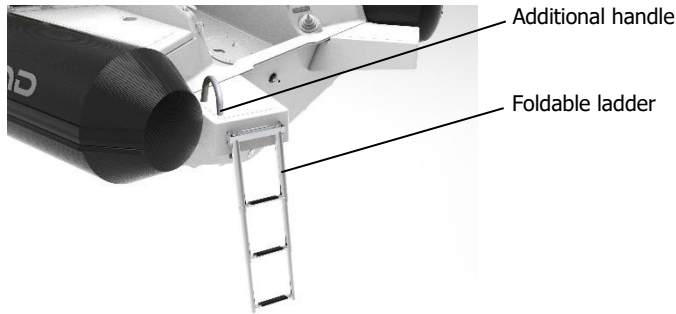
Fig. 13. Foldable ladder and handle for assistance with re-boarding.
