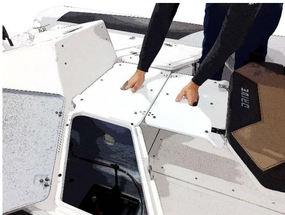
Fig. 47. How the rear sundeck should be installed.
