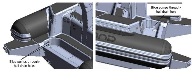
Fig. 4. Location of through-hull drain holes.
