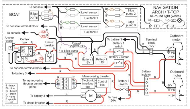
Fig. 53. Electrical schematic diagram.
