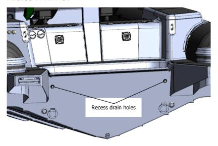
Fig. 6. Location of recess drain holes.
