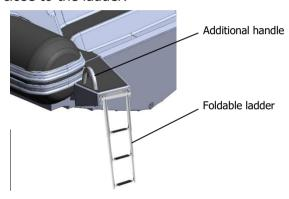
Fig. 15. Foldable ladder and handle for assistance with re-boarding.
