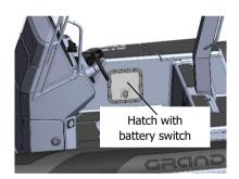
Fig. 29. Location of battery isolator switch.
