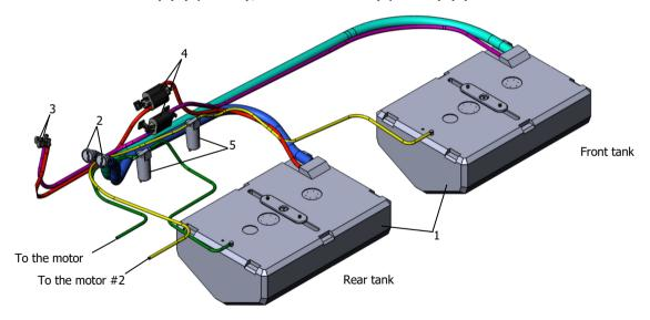
Fig. 7. The fuel system for twin motors.
