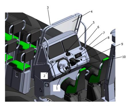
Fig. 51. Steering console components (see the list on the next page).
