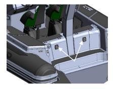
Fig. 12. Ventilation openings on the rear compartment.
