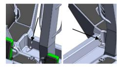
Fig.47. Bow lifting eyes, 2 positions.
