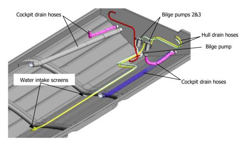
Fig. 2. The drainage system.
