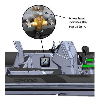
Fig. 9. 3-way fuel valve and operation guide.
