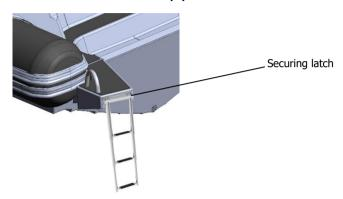
Fig. 41. Swimming platform with folding ladder.
