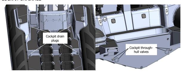
Fig. 3. Cockpit drainage.
