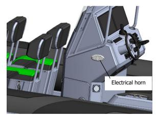
Fig. 32. Electrical horn.
