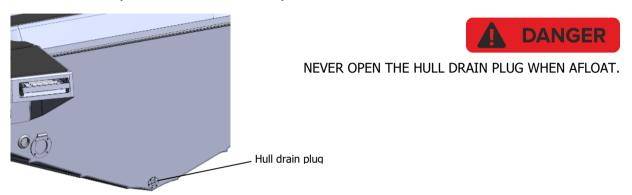
Fig. 5. Hull drainage through-hull fittings.
