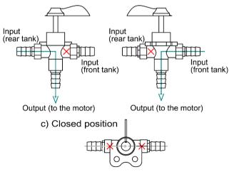
Before turn the handle to the required position, pull it up.
