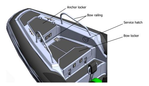
Fig. 36. Anchor locker and large bow locker compartment.
