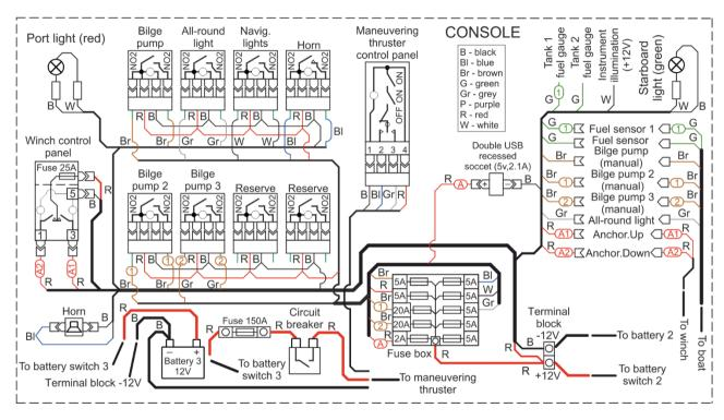
Fig. 54. Electrical schematic diagram. Steering console.
