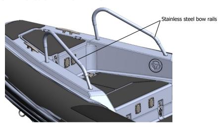
Fig. 40. Stainless steel bow rails.
