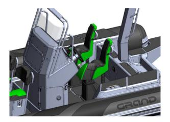
Fig. 37. Helm and passenger seats with progressive shock mitigation system.
