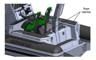
Fig. 39. Rear side rope hatches.
