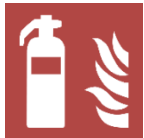
Fig. 8. Symbol of designated place of portable fire extinguisher.
