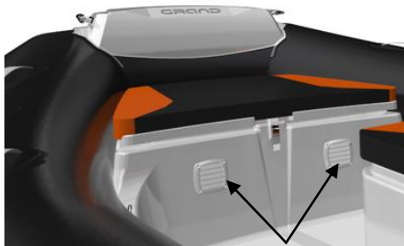
Fig. 6. Ventilation openings on the bow locker.
