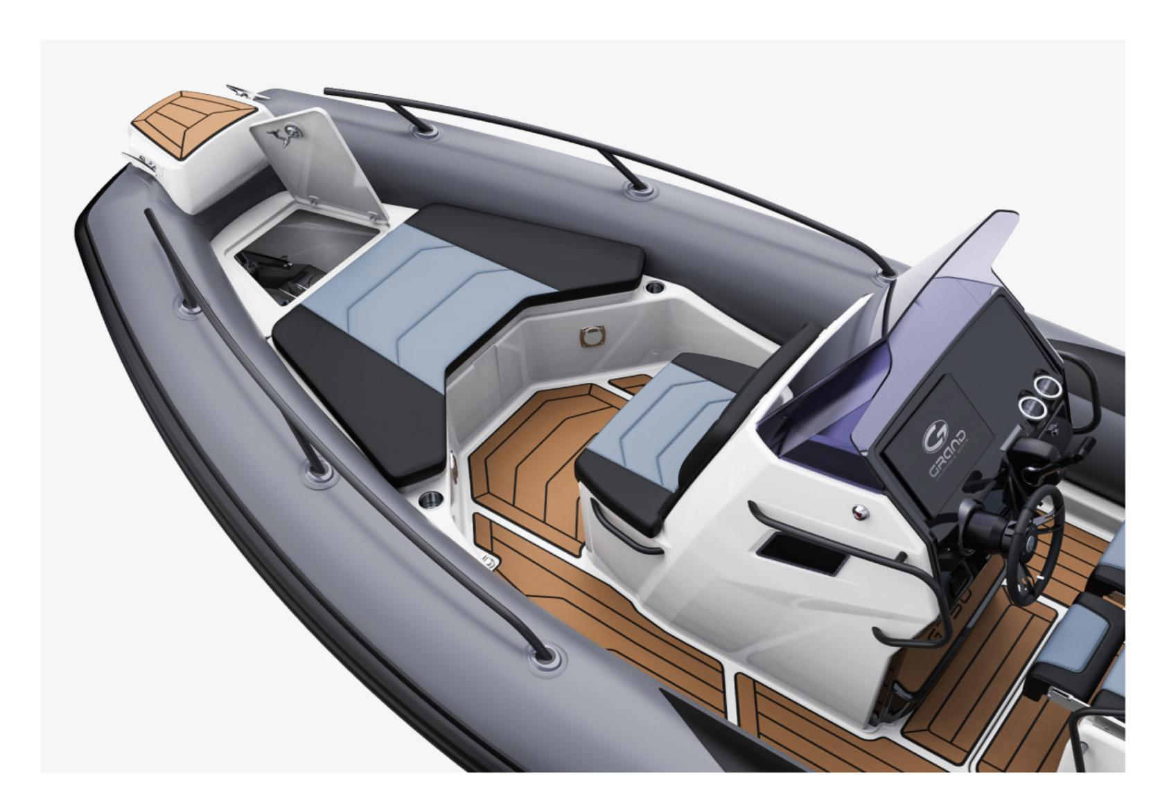
Large bow section, with two separate bow compartments – anchor and bow lockers, provides an ample sunbathing area when connected to the console seat with sundeck spacious enough to comfortably fit 2 adults. Surrounded with the safety railing and ergonomic bow step plate it creates a safe environment for the kids observation/play post.
