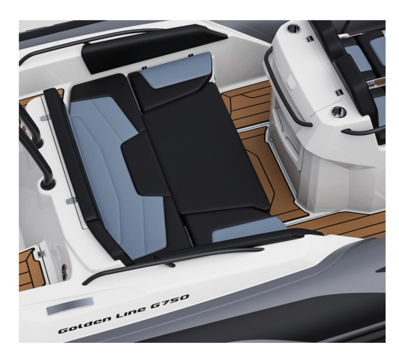
Classic U-shaped rear sofa with 2 side lockers and a generously sized middle storage compartment, all surrounded by safety handrails, it has a special feature of an open(not obstructed) passage to the rear. Enhanced by a table and fridge it creates a comfortable dining zone easily transforming into a big and delightful sunbathing area with a one-part sundeck extension.
