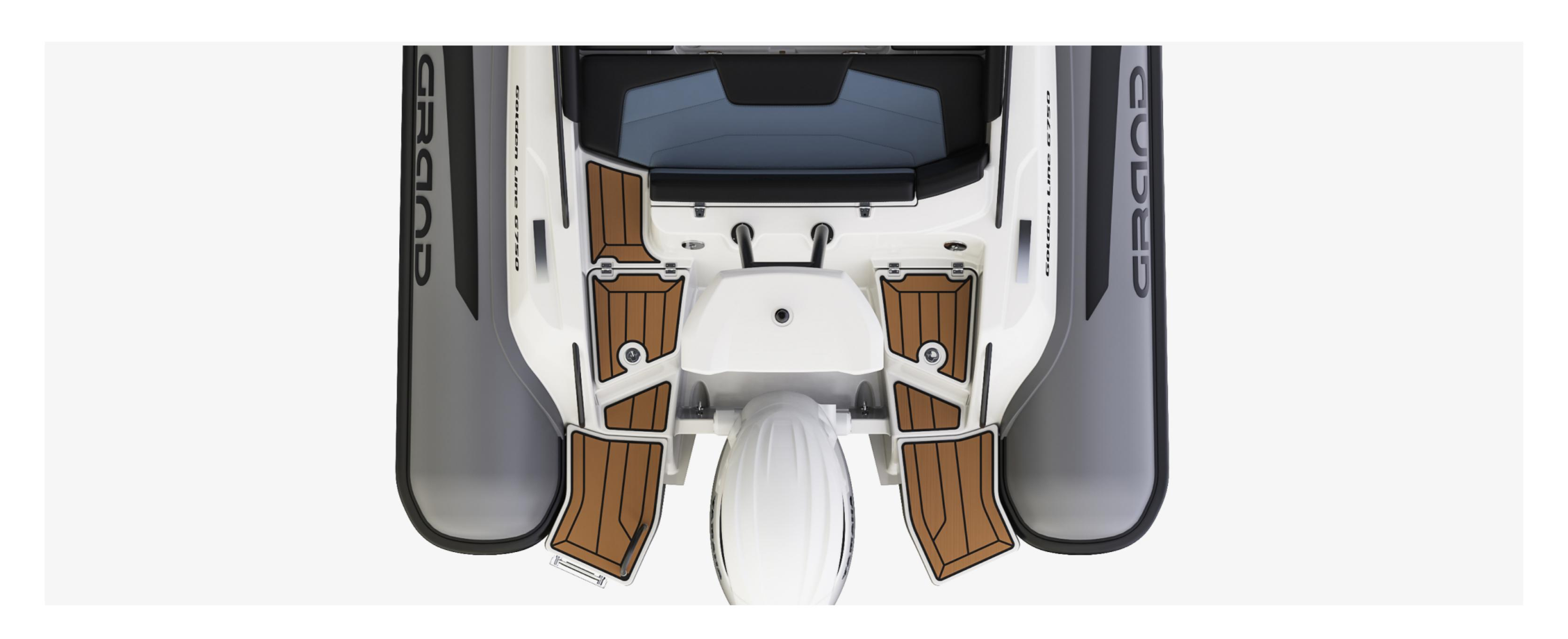
Exceptionally broad stern offers large 'wet ropes' lockers creating a staircase right on the way inside/out that, complemented with soft antiskid SeaDek flooring, makes a gradual, safe and convenient operation & walking in the rear. Traditionally, the first steps onto the boat from the water are supported by rear swimming platforms, featuring a handrail and ladder.
