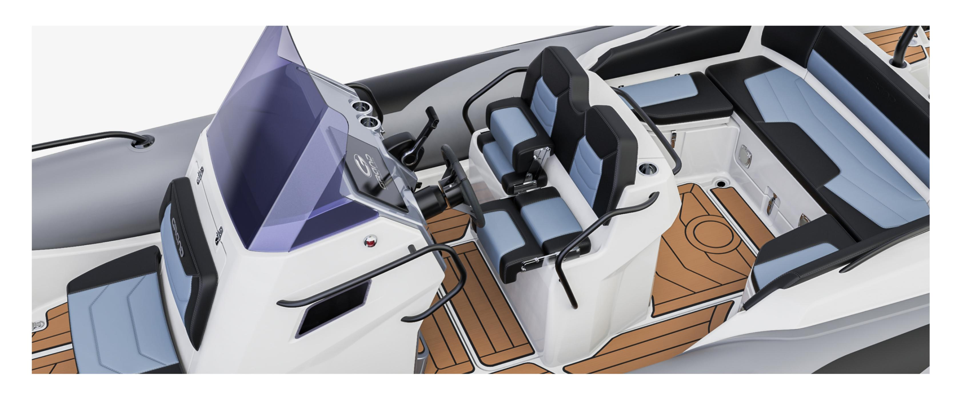
Helm & passenger bolster seat has a functional wet bar, safety handrails and lifting cushions for leaning-to-seated transition.
