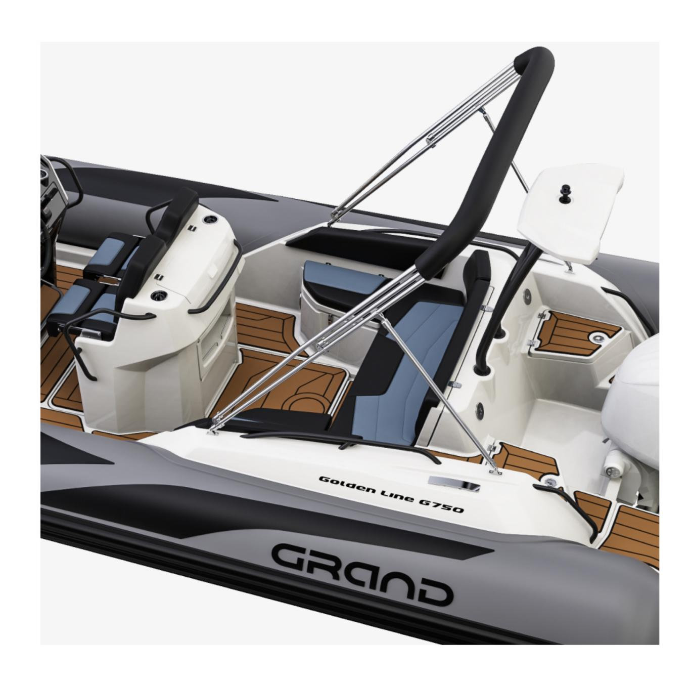
Coming as alternative to the hard-top, bimini covers slightly bigger area and should be collapsed when the boat is on the move.
