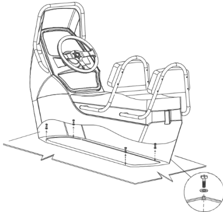
Fig. 7. Installation of steering console CS-03.
